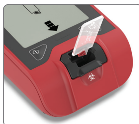
2 Place microcuvette into analyzer.
